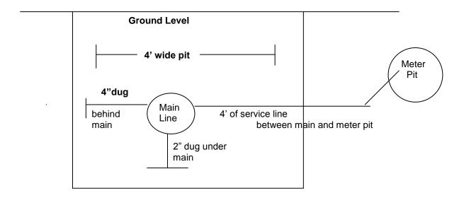
\*\* Tracer Wire to be placed from the Main Line to Meter Pit....and from the Meter Pit to the Residence.
